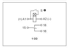
The control terminal S is activated by connection to A1 terminal via the external control contact S.
